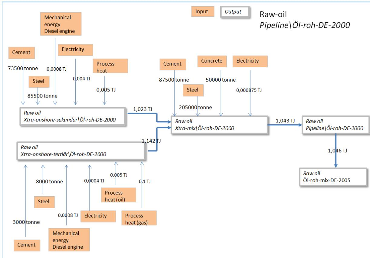
Figure 3 Process chart for oil produced in the North Sea
