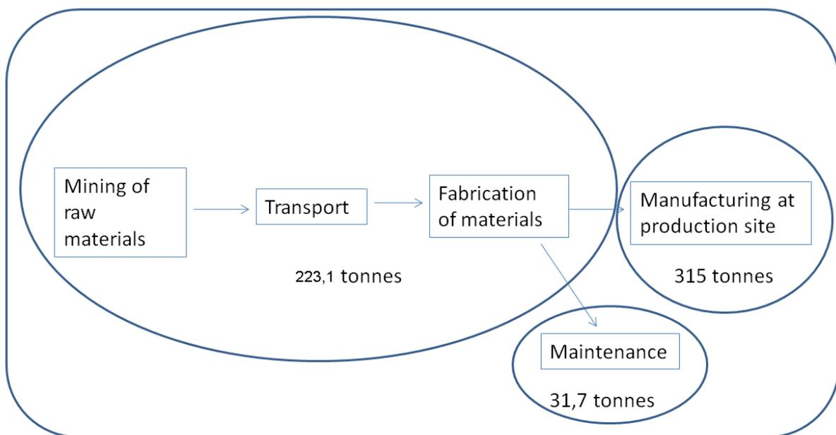
Figure 3 shows a breakdown of the estimate of CO<sub>2</sub>-equivalents arising from manufacturing and maintenance of F140 MS.
